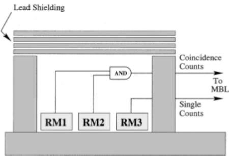
Fig. 4.— Our experimental setup. RM signifies “radiation monitor,” which in our case were Geiger tubes. We did not use the third RM, RM3. (Jackson & Welker 2001)
