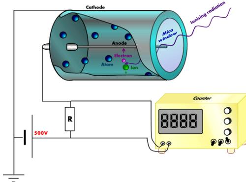
Fig. 5.— Geiger tubes such as those used in our experiment. The figure shows voltages of  $\sim 500$  V, which is similar to the voltages at which we drove our tubes.
